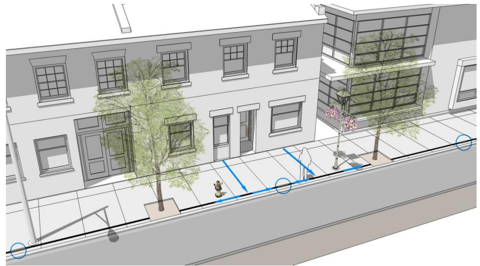
Sidewalk water into channels
