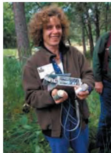
Figure 3.160. The arborsonic decay detector.
