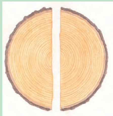
Figure 3.54. Cross section of a shear crack. The tree is split into two halves.
